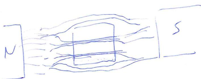
Here, there are two "thin" fluxes of magnetic field which penetrate into the material. A compromise is found between the Meissner effect and the penetration of  $\vec{B}$ . The compromise creates n form of "n" thin fluxes.
