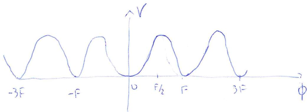
$$(\partial_t^2 - \partial_x^2)\phi = -\frac{\partial V}{\partial \phi} = -\frac{A 2\pi}{F} \sin\left(\frac{2\pi\phi}{F}\right)$$
