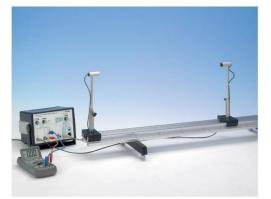
Figure 1 Measurement kit for checking the law of absorption of ultrasound in the air
